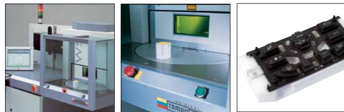
Fig.: Working area Fig.: Detail view rotary table Ø 550 mm / Ø 650 mm Fig.: Jig and workpiece (Day/Night Design)
