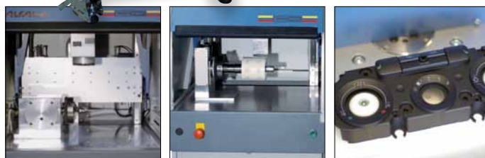
Fig.: Working chamber with dividing attachment Fig.: Automatic swing door - open Fig.: Example Day & Night Design
